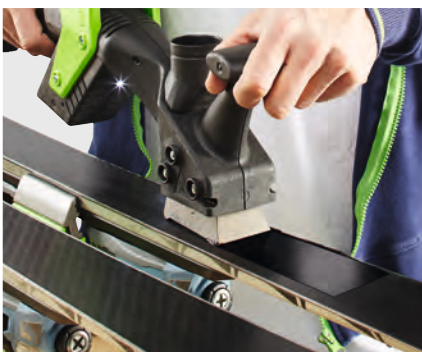
Melting head with larger contact surface
