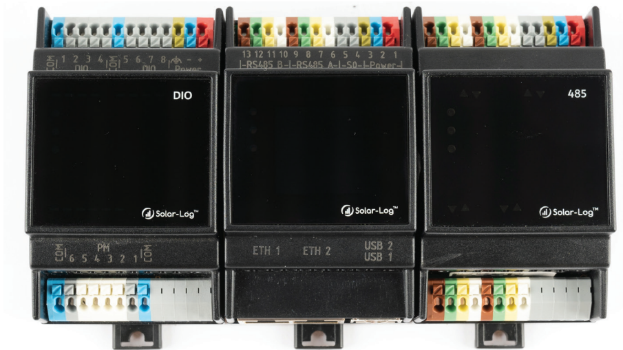
Fig.: Combination Solar-Log Base with Solar-Log MOD I/O and Solar-Log MOD 485 (Connected - front side)
