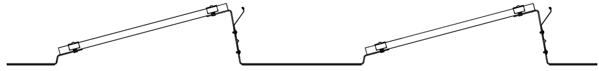
System S15 | 31.1 in. row spacing | EU18° shading angle
